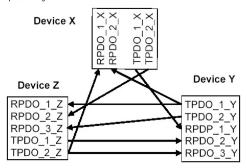
This procedure is known as PDO linking. It permits, for example, easy construction of electronic drives in which several slave axes simultaneously listen to the actual value in the master axis TxPDO.
