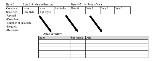
The CANopen Network Adapters are servers for the SDO, which means that at the request of a client they make data available (upload), or they receive data from the client (download).
